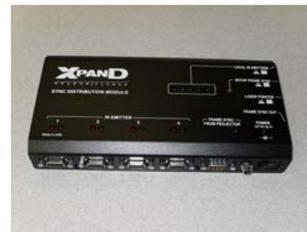
To conserve power and extend life, the distribution module activates the IR emitter arrays only if the frame sync signal is of a frequency higher than 36 Hertz and less than 80 Hertz. 3D movies use a sync rate of 48 to 72 Hertz while 2D movies use a sync rate of 24 Hertz. For this reason the unit does not have to be deactivated when 2D movies are being shown or the projector is idle.
